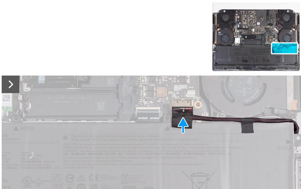
Figure 12. Connecting the battery cable
