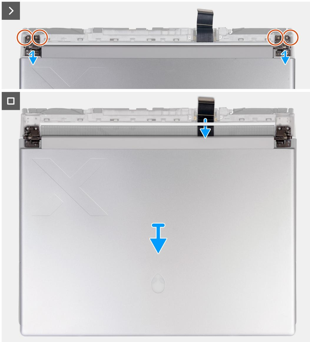
**Figure 52. Removing the display assembly**
