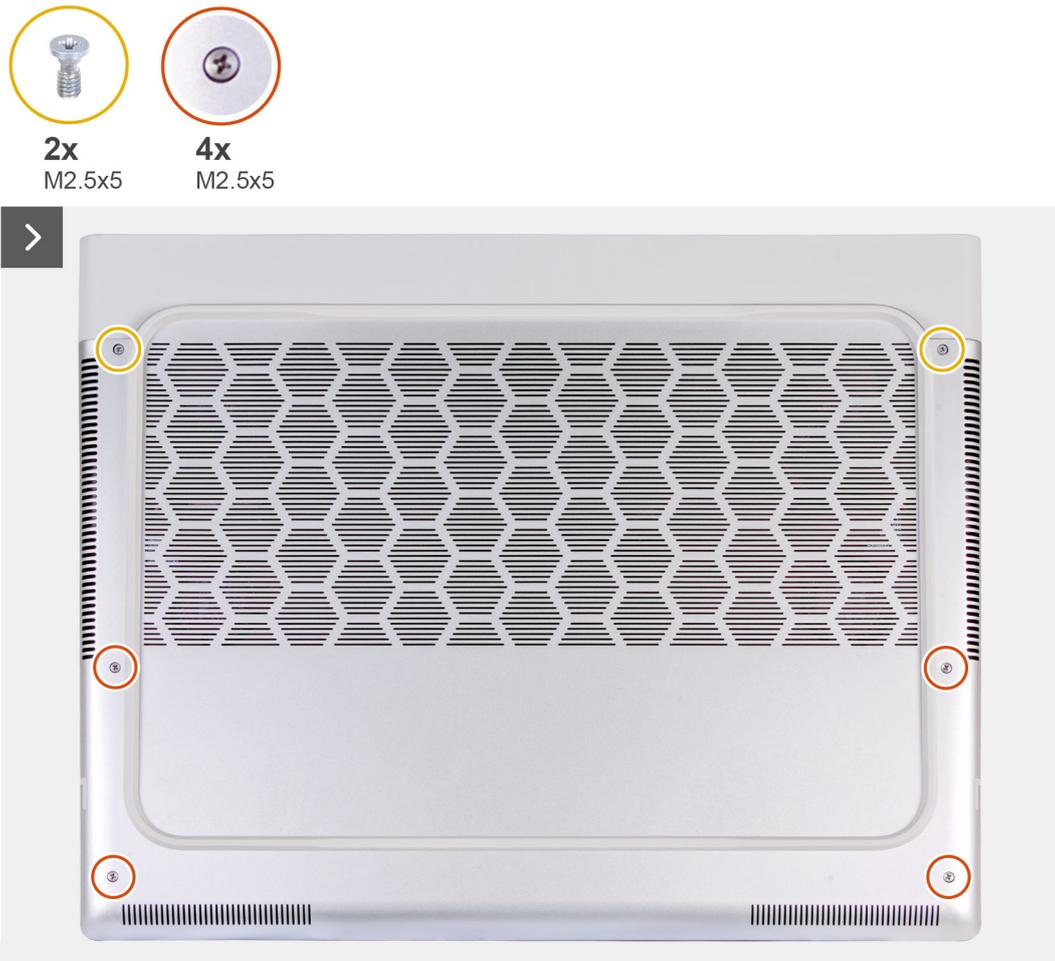
**Figure 9. Loosen the captive screws**
