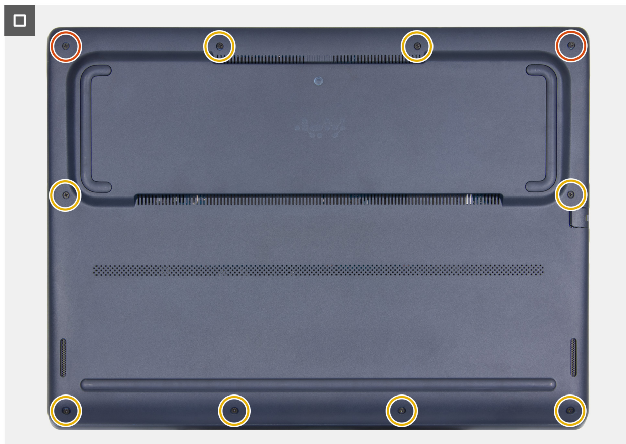
Figure 18. Installing the base cover
