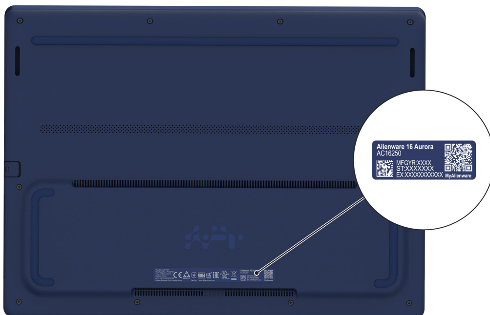
Figure 7. Service Tag/Express Service Code location
