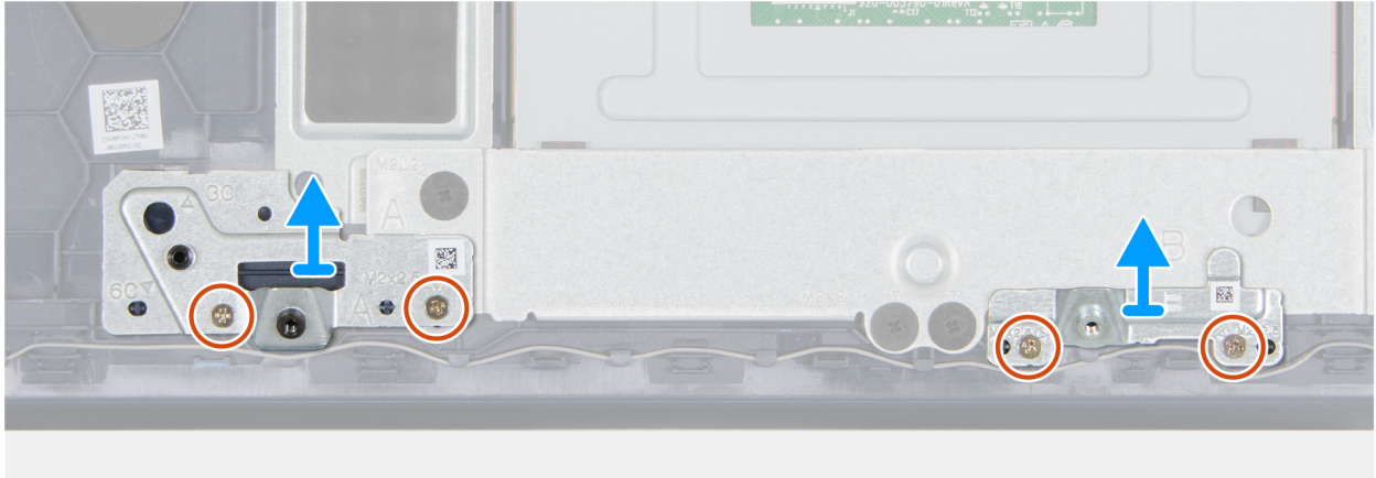
Figure 45. Removing the 6-cell battery brackets
