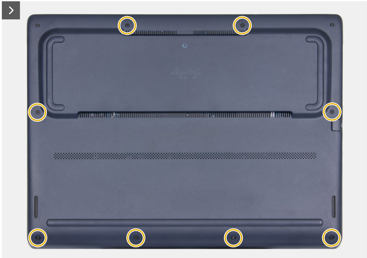
Figure 11. Removing the eight screws on the base cover
