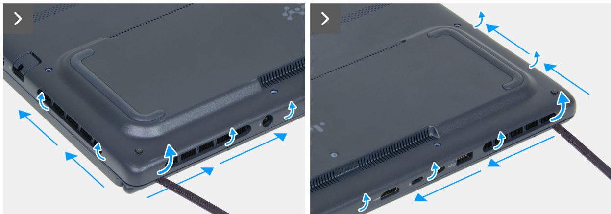
Figure 13. Inserting the scribe between the gap
