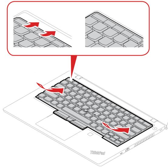
3. Slide the keyboard in the direction as shown. Ensure that the latches are secured under the keyboard frame.
