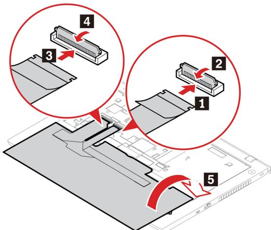
2. Insert the keyboard into the keyboard bezel as shown. Ensure that the front edge of the keyboard (the edge that is close to the display) is under the keyboard bezel.
