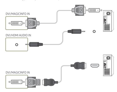
You can use the DVI port on the product as an HDMI port by using a DVI-HDMI adapter.
