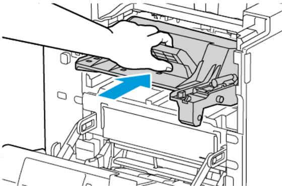
10. Slide the Toner Cartridge into the printer until it stops.
