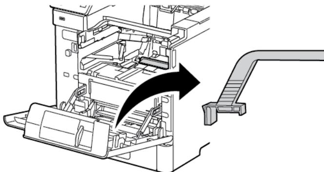
5. Remove the cleaning pad from the cleaning tool by pushing in on the two tabs. Properly recycle the used cleaning pad.
