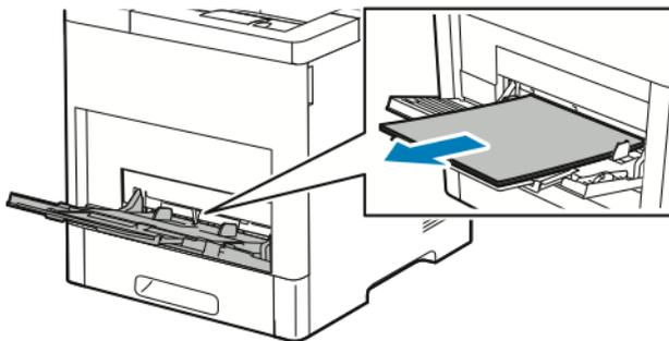
2. Grasp both sides of the Bypass Tray, then pull it straight out of the printer.
