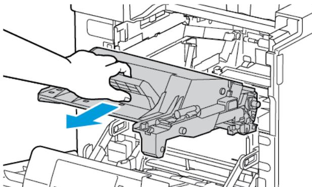
**4. Remove the cleaning tool from inside the Front Door.**
