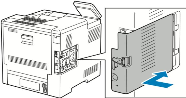
7. To latch the cover, swing the handle toward the front of the printer, then push the handle in until it clicks into the locked position.
