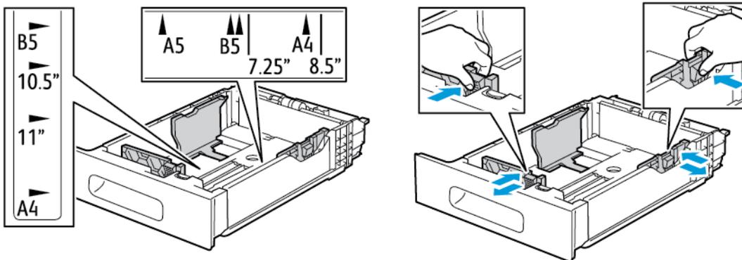
4. Load envelopes in the trays with the flaps closed, flap-side down, and the short edge leading into the printer.
