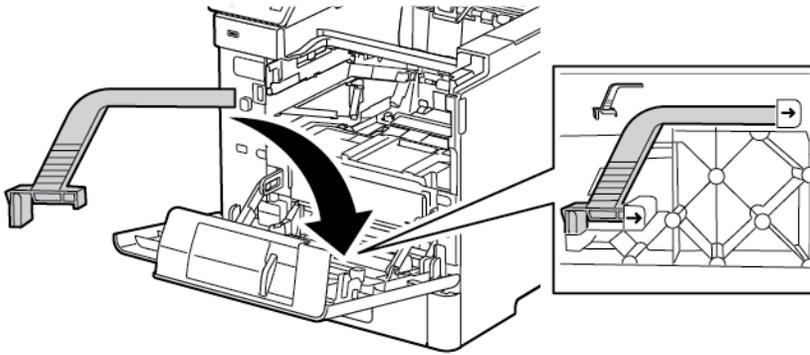
9. Slide the Drum Cartridge into the printer until it stops.
