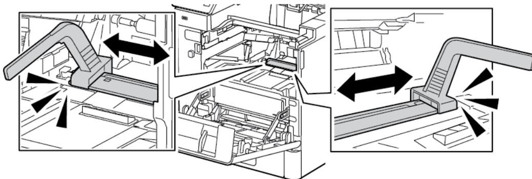
8. Replace the cleaning tool into its storage location inside the Front Door.
