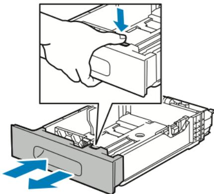
4. To extend the tray for longer paper, hold the back of the tray with one hand. With the other hand, press the release latch at the front of the tray, then pull the ends outward until they latch.
