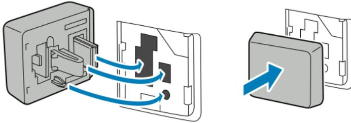
6. Place the left-side cover into place, then slide it toward the front of the printer.
