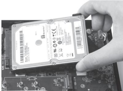
4. Secure the installed drive with a thumb screw.
