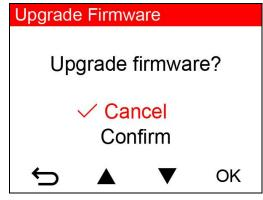
WARNING: NEVER remove the power cord or the microSD memory card while the firmware is being upgraded.
