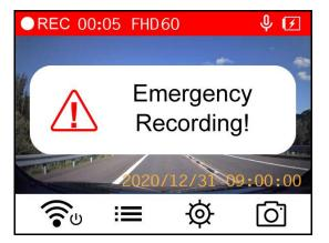
**G-Sensor Event Recording:** During video recording, the DrivePro will automatically activate Emergency Recording mode when detecting a collision.
