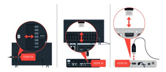
First disconnect and reconnect the power cables and HDMI cables on the back of your TV or the One Connect (OC) Box, then unplug the power cable and plug it back into the wall outlet.
