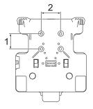
1 Height: 1.18 in. (30 mm)2 Width: 1.5 in.(38.1 mm)
