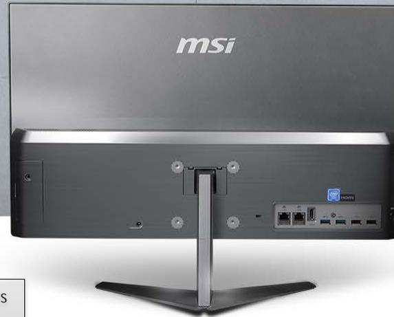
PRO 24X can be mounted to the wall in your office/ home, thanks to its supports of VESA-mount standards, which makes the PC completely invisible on a desk.
