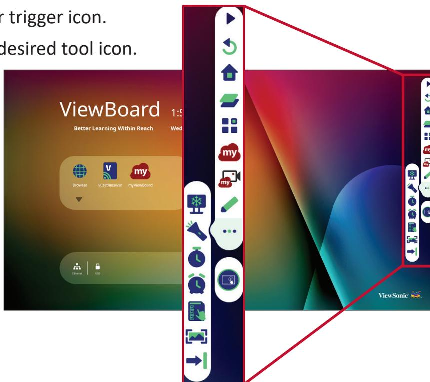
**NOTE:** The default toolbar setting is to be available for all input sources; however, users can go to: **Settings > Preference > Toolbar setting** to adjust the options: (1) available for all input sources, (2) hide the toolbar for all input sources.
