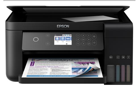
This next generation, cartridge-free 3-in-1 comes with a range of connectivity options, double-sided printing and 6.1cm LCD screen.
