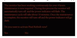
After every 4 hours of cumulative operation, the screen compensation correction and image residue elimination function will automatically run when the display is turned off, or has been in standby for 2 hours.
