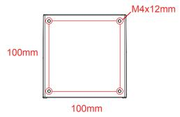
Specification of wall hanger screws: M4\*12mm
