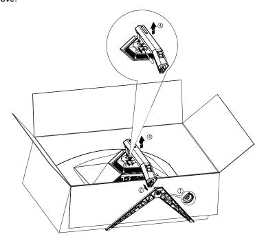
Specification for base screw: M8\*35 mm (effective thread 10 mm)
