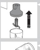
9 Carefully remove the chopper lid and the blade unit (fig. 18).
