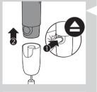
9 Press the release button to remove the motor unit from the whisk coupling unit.
