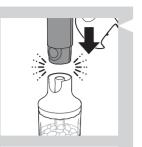
4 Attach the motor unit onto the chopper lid ("click").
