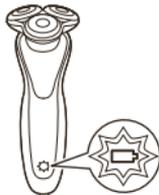
**Quick charge:** After approx. 5 minutes of charging, the shaver contains enough power for one shave. At that moment, the battery charge indicator stops flashing quickly and starts flashing slowly.
