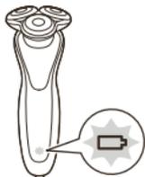
When the battery is almost empty, the battery charge indicator flashes orange. At this point there is enough energy left for one shave.
