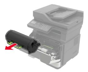
**3** Remove the used imaging unit.
