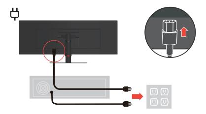
11. Connect the cables with cable clip.
