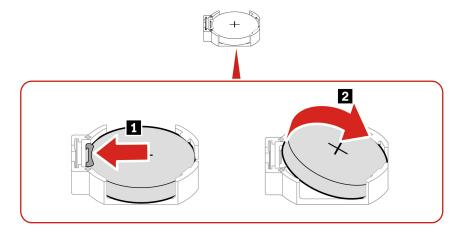
Note: After installing a new coin-cell battery, reset the system date and time in the UEFI BIOS menu.
