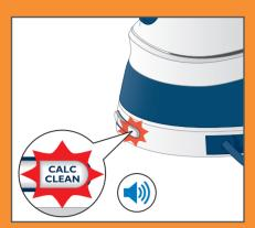
Perform descaling once the descaling light flashes and the appliance beeps.
