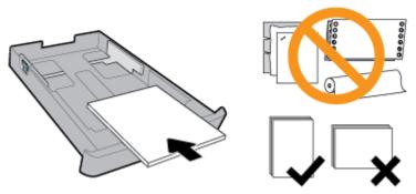
Make sure the stack of paper is aligned with the appropriate paper size lines on the front of the tray. In addition, make sure the stack of paper does not exceed the stack height marking on the right edge of the tray.
