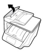
Pull any jammed paper out of the rollers.
