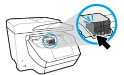
Make sure that the color-coded letter on the cartridge matches that on the slot.
