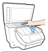
**ACCITION:** Use only glass cleaner to clean the scanner glass. Avoid cleaners that contain abrasives, acetone, benzene, and carbon tetrachloride, all of which can damage the scanner glass. Avoid isopropyl alcohol because it can leave streaks on the scanner glass.
