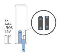
Remove the batteries if you are not using the remote control for a long time.
