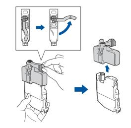
Quickly shake just the black ink cartridge horizontally 15 times as shown, before inserting it into the machine.
