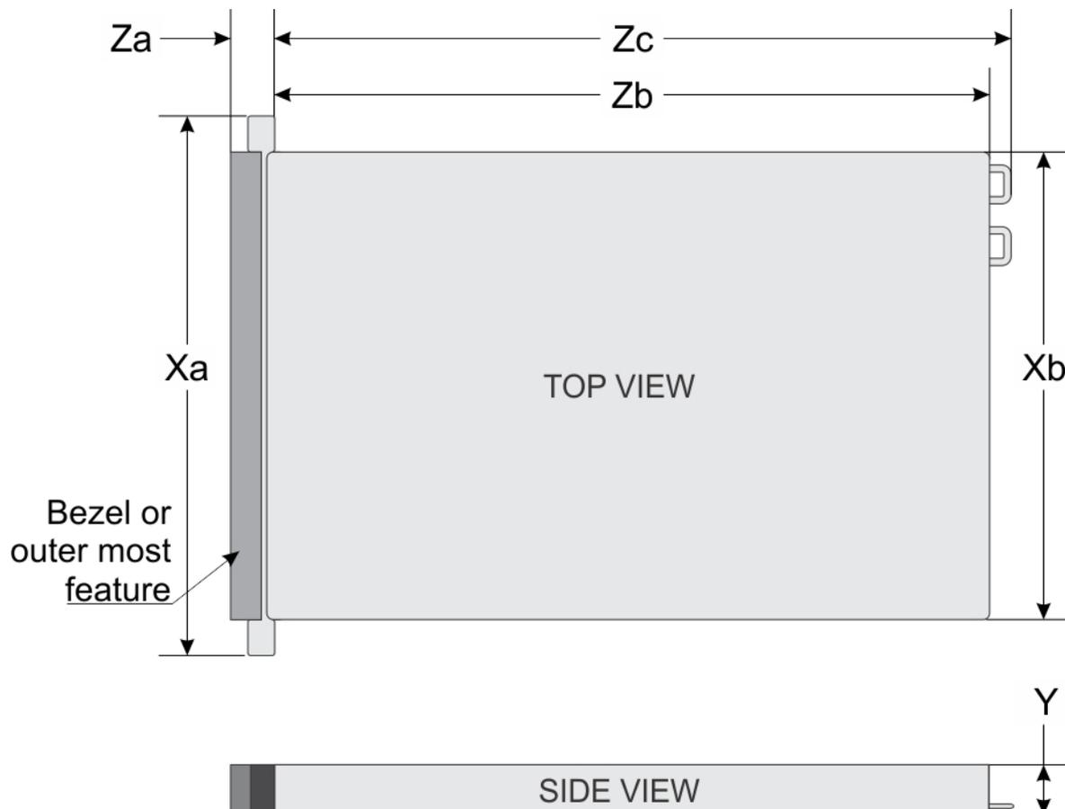
Figure 1. Dimensions of the Dell EMC PowerEdge R440 system
