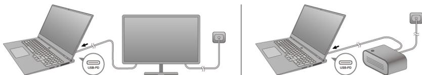
In another scenario, if you carry your computer around without the included ac power adapter, you may use a capable USB-C charger to provide power through the rear USB-C port. In both scenarios, the output power of a USB-C charger or the USB-C port on a dock or display should be at least 20 V and 2.25 A in order to provide power to your computer. The following table lists the charging capability of a USB-C port on a charger or an external device based on its maximum output power.
