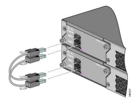
**Note** When you connect the FlexStack cable to the STACK 1 port, the tab should be above the connector. When you connect the FlexStack cable to the STACK 2 port, the tab should be below the connector.
