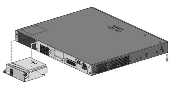
**Step 3** Secure the screws on each side of the module.
