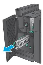
4. Pull the green handle of the stapler unit toward you and rotate it upward. Push the handle in to lock it in the open position.
