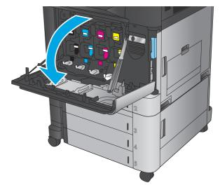
Grasp the handle of the used imaging drum and pull out to remove it. Grasp the blue handle on the top of the imaging drum to support it.
