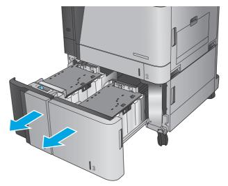
On each side, adjust the paper-size lever to the correct position for the paper you are using.
