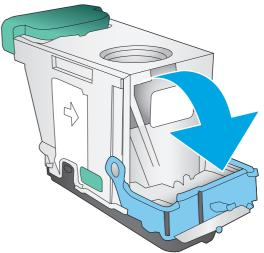
Insert the staple cartridge. Press down on the top of the staple cartridge until it clicks into place.
