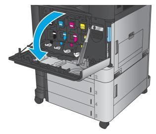
2. Grasp the handle of the used toner cartridge and pull out to remove it.
