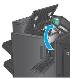
If paper is jammed in the bottom of the holepunch unit, carefully remove it.
