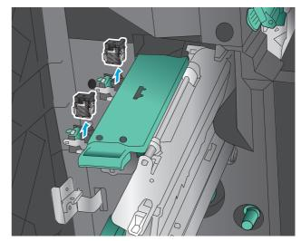
Press down on the jam-release at the back of the saddle-staple cartridge, push up on the plate at the front of the cartridge, and then remove any jammed staples.
