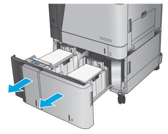
2. Remove the paper from the trays and discard any damaged sheets.
