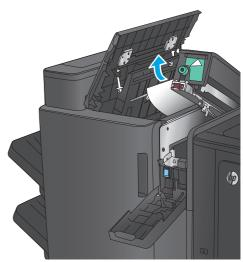
**8. Hole punch models only:** Close the hole-punch unit.
