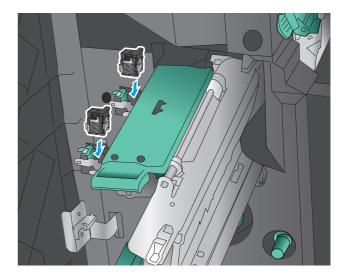
Pull the handle of the staple cartridge unit toward you and rotate it downward to its original position. Lock it into position by pushing in the handle.
