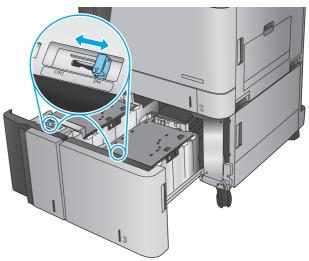
3. Load full reams of paper into each side of the tray. The right side holds 1,500 sheets of paper. The left side holds 2,000 sheets of paper.
