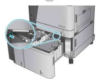
**4.** If jammed paper is in the feed area, pull it down to remove it.
