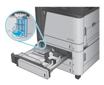
Load paper into the tray. Check the paper to verify the guides lightly touch the stack, but do not bend it.
