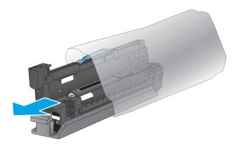
4. Align the imaging drum with its slot, and then insert the imaging drum into the product. The protective cover on the bottom of the drum automatically slides off as the imaging drum is inserted. Recycle this cover with the used imaging drum.
