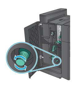
**14.** Press the large jam-release knob, and then turn it clockwise.
