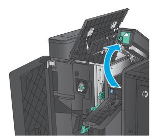
**6. Hole punch models only:** If paper is jammed in the bottom of the hole-punch unit, carefully remove it.
