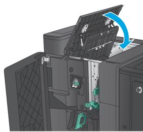
10. Move the lower jam-release lever to the right, and then remove any paper. Move the lower jam-release handle to the left.
