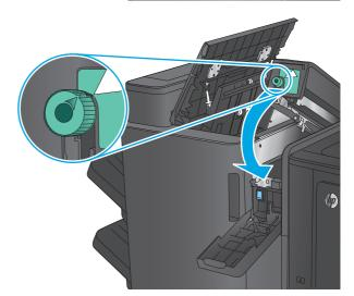
**9. Hole punch models only:** Close the hole-punch door.
