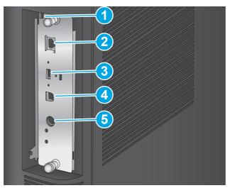
1 Slot for a cable-type security lock
