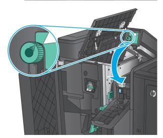
**8. Hole punch models only:** Close the hole-punch door.
