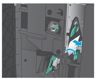
11. Move the upper jam-release lever to the right, and then remove any paper. Move the upper jam-release handle to the left.
