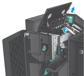
**7. Hole punch models only:** Close the hole-punch unit.
