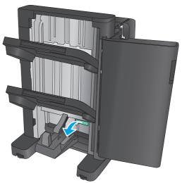
**13.** Turn the small jam-release knob counterclockwise.
