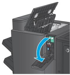
**3. Hole punch models only:** Turn the knob to align the arrows.
