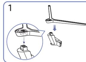
Put the stand base onto the stand neck as the direction shown in the figure. Check that the stand neck is firmly connected.
