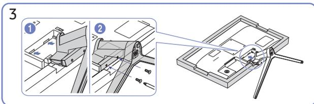
Place a soft cloth over the table to protect the product and place the product onto the cloth so that the front of the product is facing downwards. Push the assembled stand into the main body in the direction of the arrow as shown in the figure. Tightly fasten the connecting screw at the bottom of the main body.
