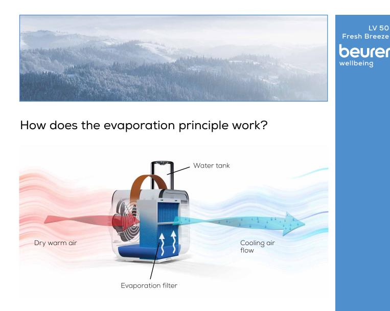
The air fan draws in the dry warm air from the room, which then comes into contact with the evaporation filter, which is saturated with water. The contact between the air flow and the damp filter surface causes the water to evaporate. The ambient air absorbs the humidity, and the thermal energy required for the evaporation process is extracted from the ambient air. There is a noticeable drop in the temperature of the ambient air.
