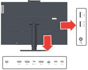
3. Engineering port only for specialist test usage. Do Not plug in any connector of this port to prevent malfunction of the monitor or any electrical accident caused.
