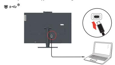
7. For computer in USB type C-A connecting. **Note:** Monitors sold in NA include a USB type C-A cable
