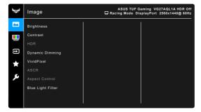
Brightness: The adjusting range is from 0 to 100.
