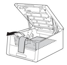
Remove the orange packing piece from each drum and toner cartridge assembly.
