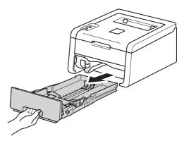
While pressing the green paper-guide release lever ①, slide the paper guides to fit the paper size you are loading in the tray. Make sure the guides are firmly in the slots.
