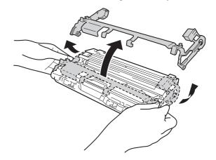
Using both hands, hold each drum and toner cartridge assembly level, and gently shake it from side to side several times to distribute the toner evenly inside the assembly.
