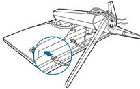
• Using the input/output port cover: the cover can be attached or detached.
