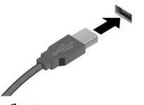
Connect USB-compatible devices, such as a USB keyboard, USB mouse, USB storage device, or USB printer.
