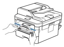
4. Using both hands, put one full sheet of paper in the manual feed slot until the front edge touches the paper feed roller. When you feel the machine pull it in, let go.
