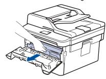
4. Push down the green lock lever, and then take the toner cartridge out of the drum unit as shown in the illustration.
