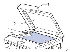
3. In the ADF unit, clean the white bar (1) and the scanner glass strip (2) underneath it with a soft lint-free cloth moistened with water.
