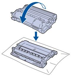
9. Use the numbered markers next to the drum roller to find the mark on the drum. For example, a dot in column 2 on the check sheet means that there is a mark in drum region "2".
