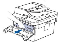
8. Turn the drum unit as shown in the illustration. Make sure that the drum unit gear is on the left side.
