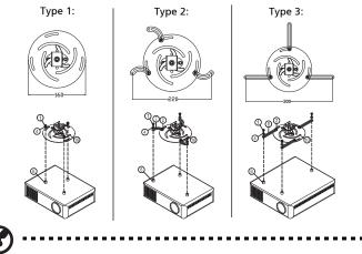
**Note:** It is recommended that you keep a reasonable space between the bracket and the projector to allow for proper heat distribution.
