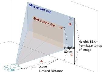
**Note:** Remind as below figure, the space of 89 cm height is required when located at 2 m distance.
