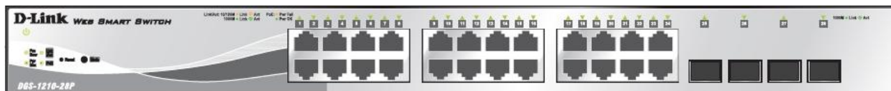
Figure 1.9 – DGS-1210-28P Front Panel
