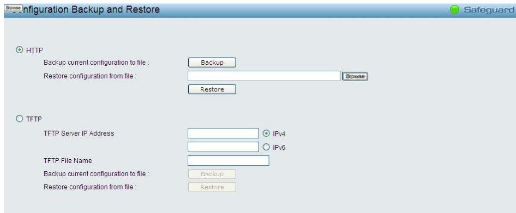
Figure 4.13 – Tool Menu &gt; Configure Backup and Restore
