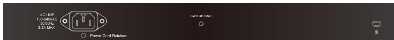
Figure 1.14 – DGS-1210-52P Rear Panel
