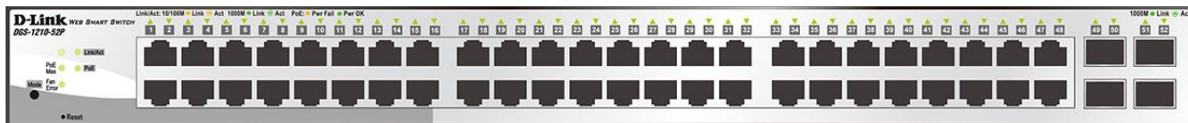
Figure 1.13 – DGS-1210-52P Front Panel
