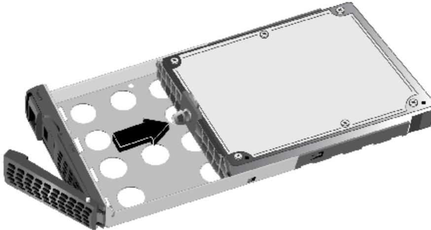
6. Remove the old HDD from the mounting bracket.
