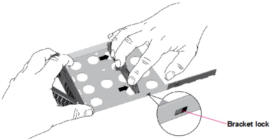
The mounting bracket stops when it hits the bracket lock.
