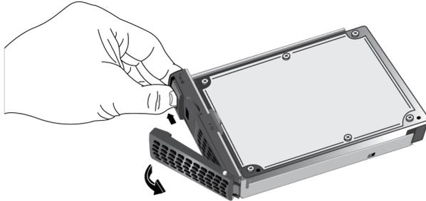
5. While holding the disk tray release latch, pull out the mounting bracket and slide the bracket down the tray.
