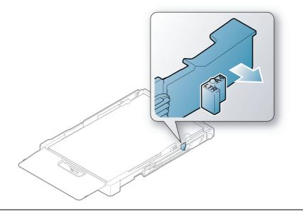
If you want to change the size to A4, first move the paper width guide to left and rotate the lever counterclockwise. If you force the lever, it could damage the tray.
