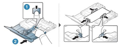
For paper longer than Legal-sized, press and unlatch the guide lock in the tray, pull the tray out manually. Then adjust the paper length guide and paper width guide.
