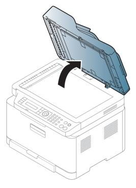
2 Place the original face down on the scanner glass. Align it with the registration guide at the top left corner of the glass.
