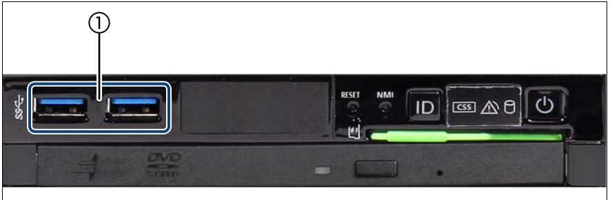
Figure 8: Front side connectors 2.5-inch version
