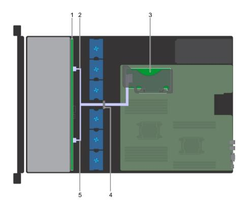
Figure 97. Cable routing -  $8 \times 3.5$  inch drive backplane with internal PERC riser
