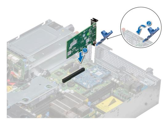
Figure 75. Installing expansion card on system board
