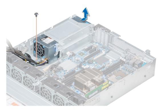
Figure 110. Removing non-redundant cabled AC PSU
