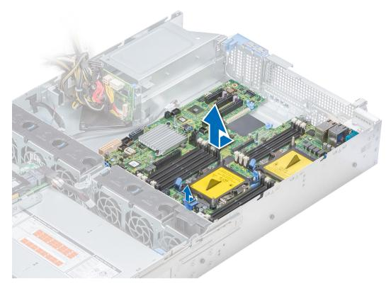
Figure 119. Removing the system board
