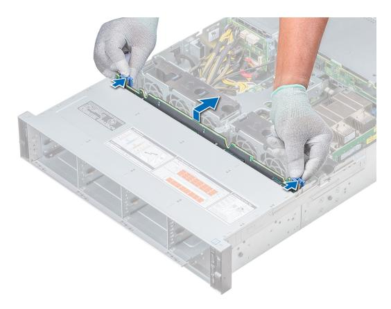
Figure 92. Removing drive backplane
