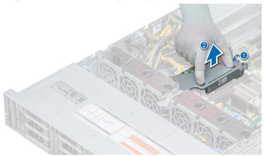
Figure 32. Removing internal PERC riser
