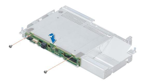
Figure 95. Installing 3.5 inch rear drive backplane
