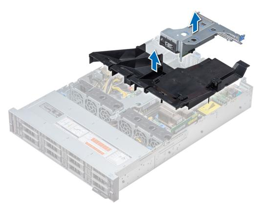
Figure 26. Removing air shroud
