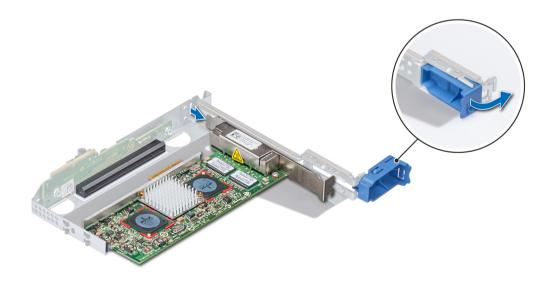
Figure 61. Removing expansion card from full height X1 riser
