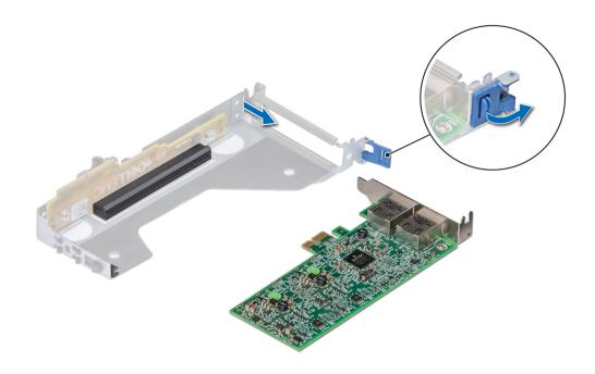
Figure 60. Removing expansion card from low profile riser
