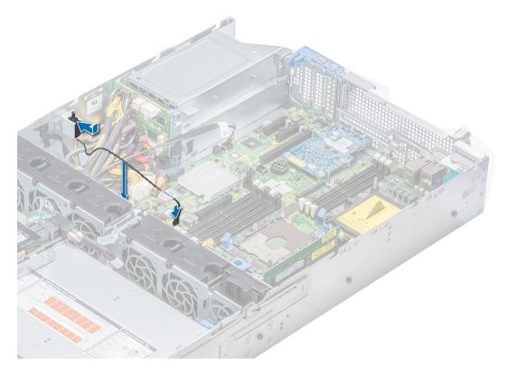
Figure 39. Installing intrusion switch
