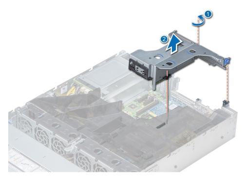
Figure 79. Removing butterfly riser
