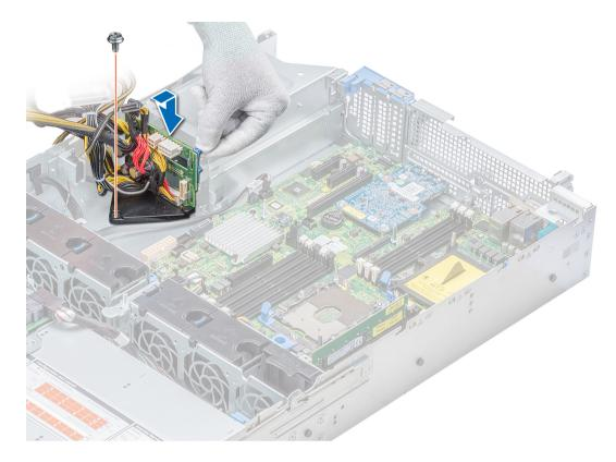
Figure 113. Installing power interposer board
