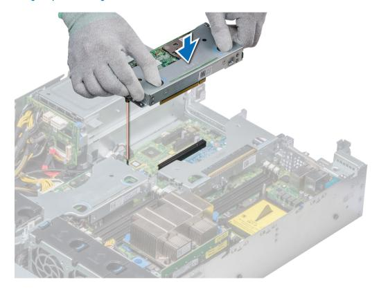
Figure 81. Installing low profile riser left
