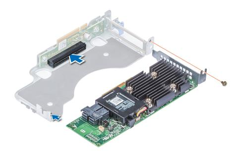
Figure 37. Installing PERC card into internal PERC riser
