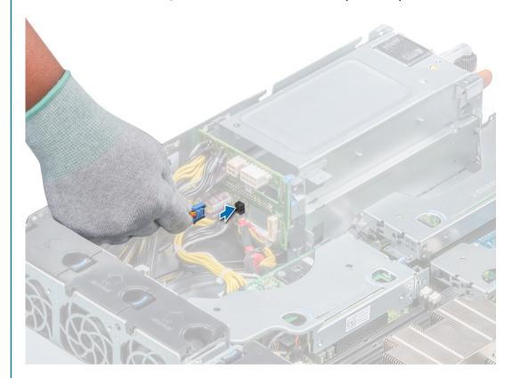
Figure 31. Connecting fan cable to PIB connector
