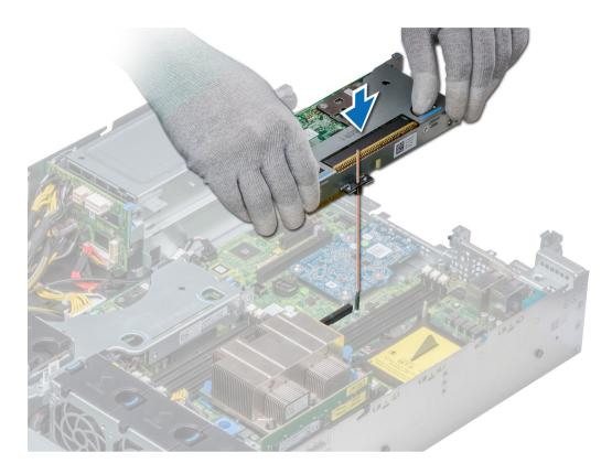
Figure 76. Removing low profile riser right
