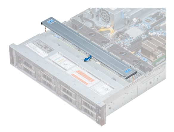
Figure 23. Installing backplane cover
