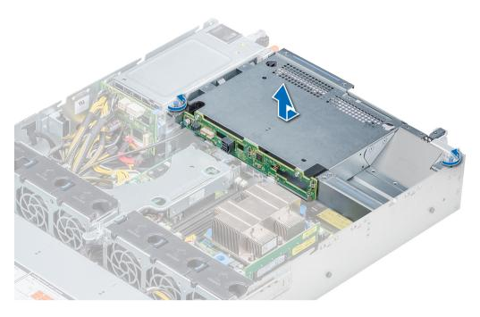
Figure 100. Removing the rear drive cage
