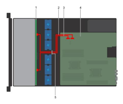
Figure 99. Cable routing - 8 x 3.5 inch drive backplane
