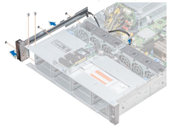
Figure 114. Removing left control panel
