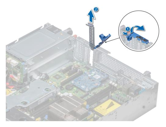
Figure 74. Removing the filler bracket
