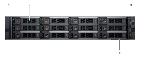
Figure 2. Front view of  $12 \times 3.5$  inch drive system
