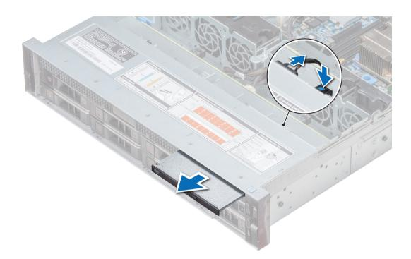
Figure 104. Removing optical drive
