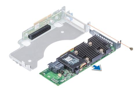
Figure 36. Removing PERC card from internal PERC riser
