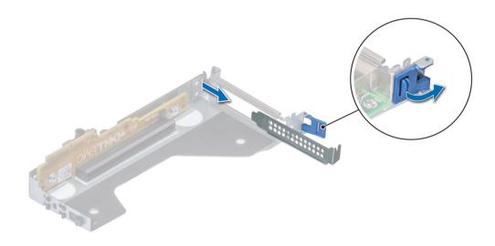
Figure 66. Removing filler bracket for low profile riser
