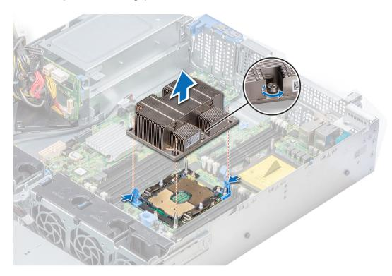
Figure 53. Removing processor and heat sink module
