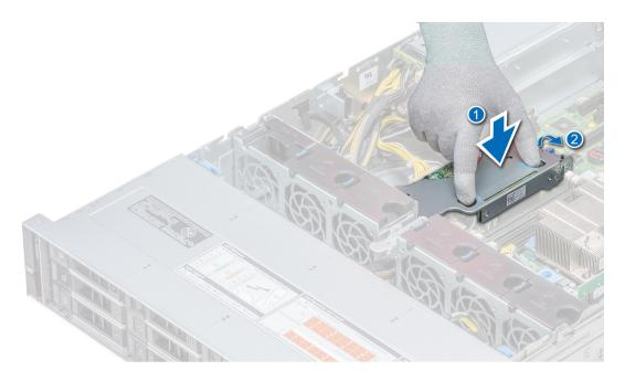
Figure 35. Installing internal PERC riser
