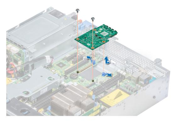
Figure 86. Removing LOM riser card
