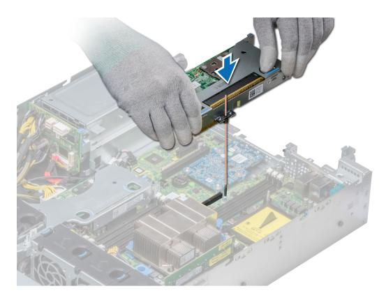
Figure 80. Installing low profile riser right
