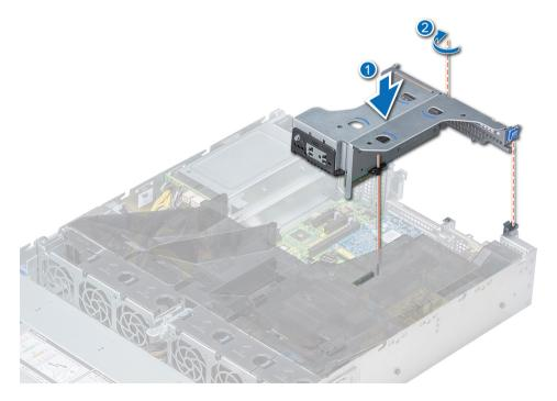
Figure 83. Installing butterfly riser
