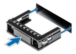
Figure 41. Installing a drive blank
