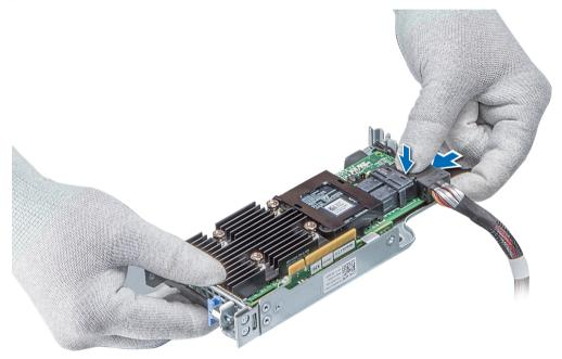
Figure 34. Connecting the cable to internal PERC riser
