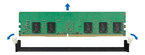
Figure 51. Removing a memory module
