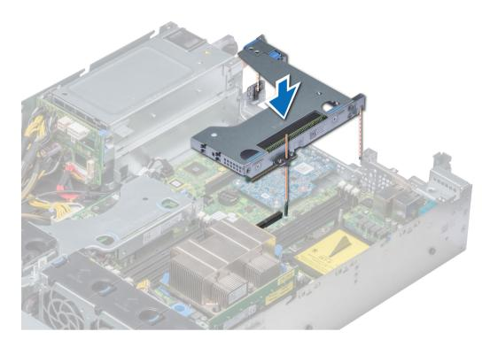
Figure 82. Installing full height X1 riser
