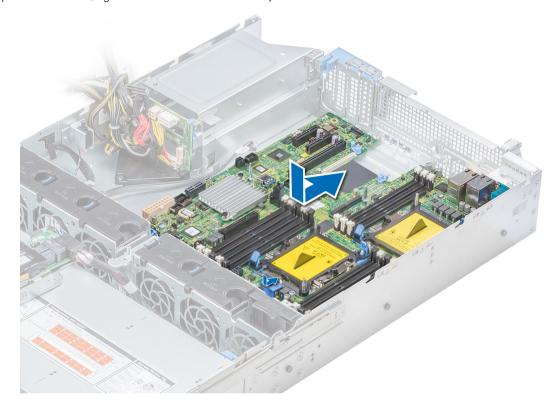
Figure 120. Installing system board
