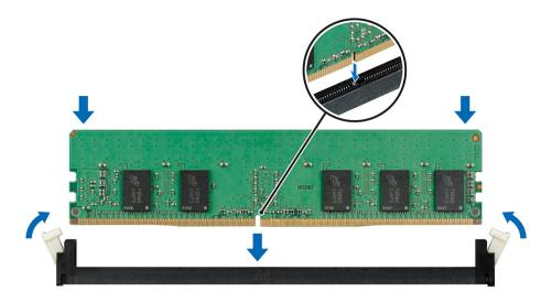
Figure 52. Installing a memory module
