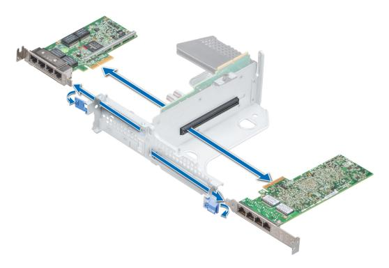
Figure 62. Removing expansion card from butterfly riser
