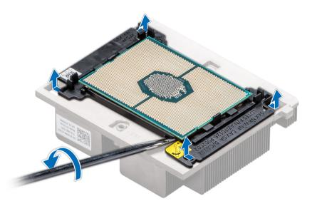
Figure 54. Loosening the processor bracket
