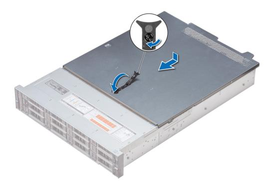
Figure 21. Installing system cover
