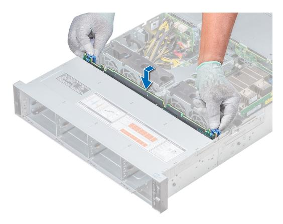
Figure 93. Installing drive backplane
