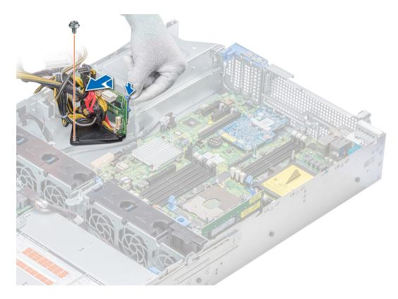
Figure 112. Removing power interposer board
