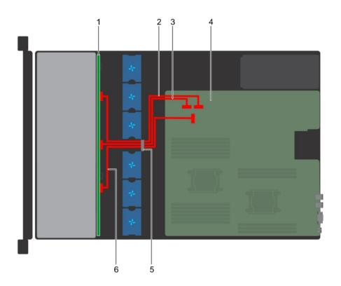
Figure 98. Cable routing -  $12 \times 3.5$  inch drive backplane
