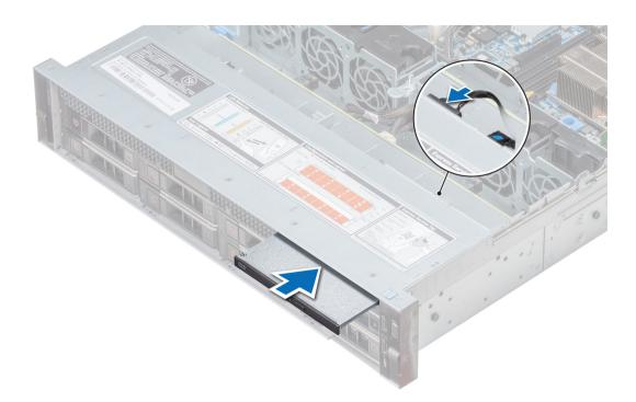
Figure 105. Installing the optical drive
