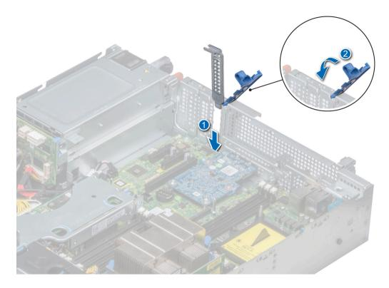
Figure 73. Installing the filler bracket
