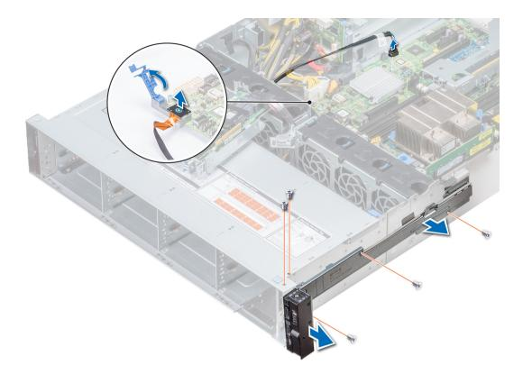
Figure 116. Removing right control panel
