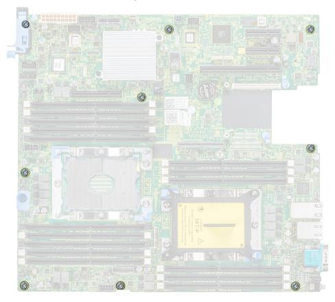
Figure 118. System board screws
