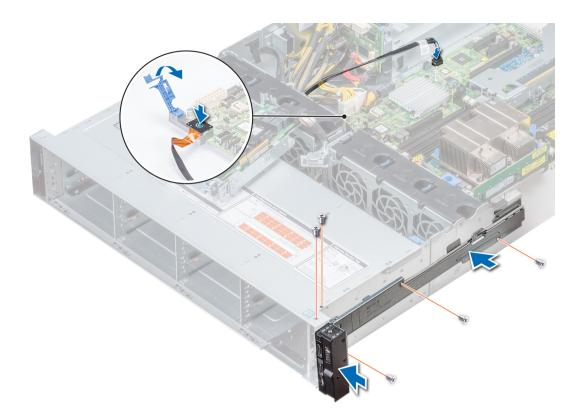
Figure 117. Installing right control panel
