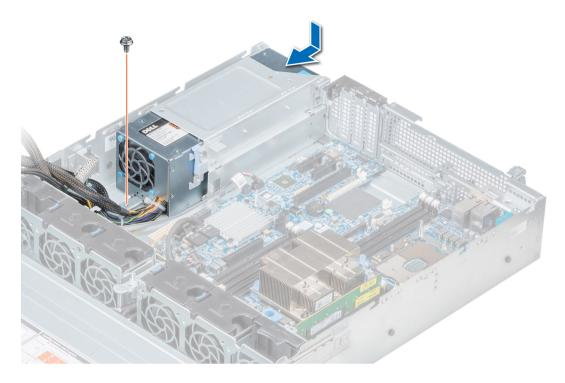
Figure 111. Installing non-redundant cabled AC PSU
