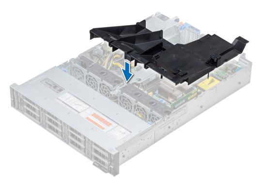
Figure 27. Installing air shroud
