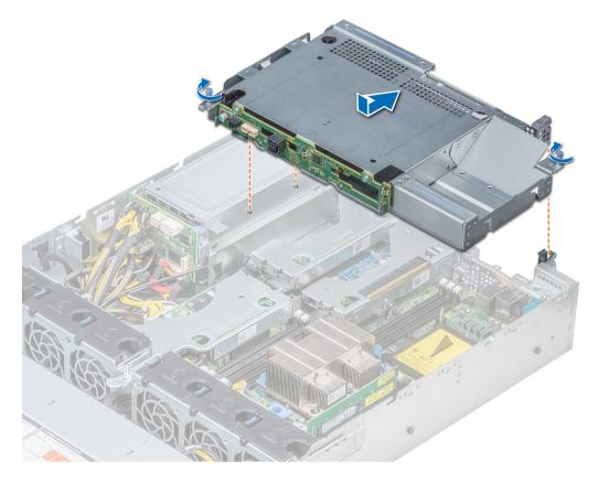
Figure 101. Installing the rear drive cage
