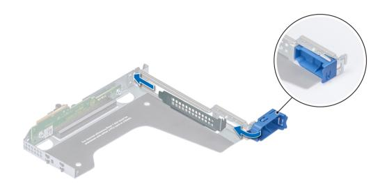
Figure 64. Installing filler bracket for full height X1 riser
