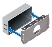
Figure 107. Installing a power supply unit blank
