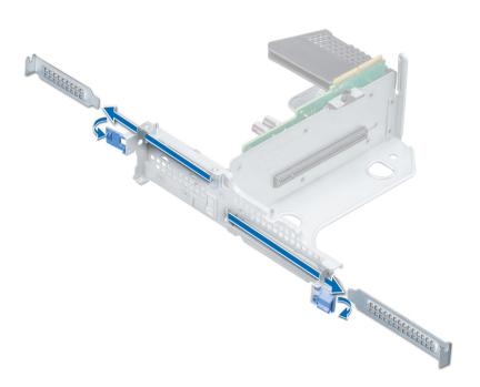
Figure 68. Removing filler bracket for butterfly riser
