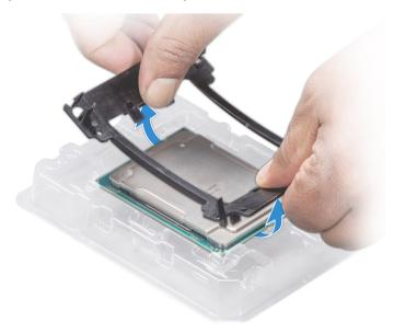
Figure 55. Removing the processor bracket
