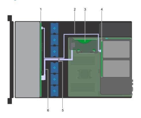
Figure 96. Cable routing -  $12 \times 3.5$  inch drive backplane and  $2 \times 3.5$  inch rear drive backplane with internal PERC riser
