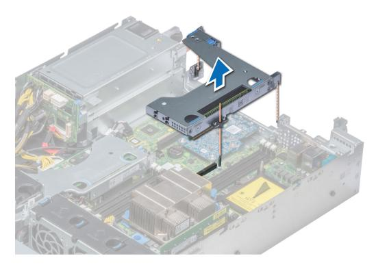
Figure 78. Removing full height X1 riser
