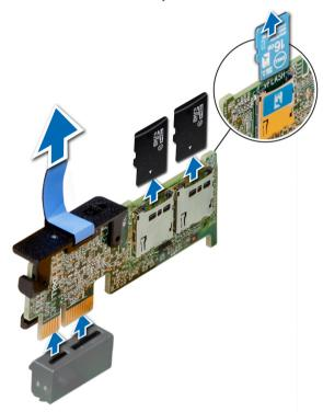
Figure 84. Removing the optional IDSDM/vFlash card
