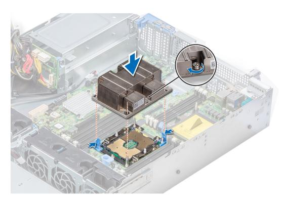
Figure 59. Installing the processor and heat sink module
