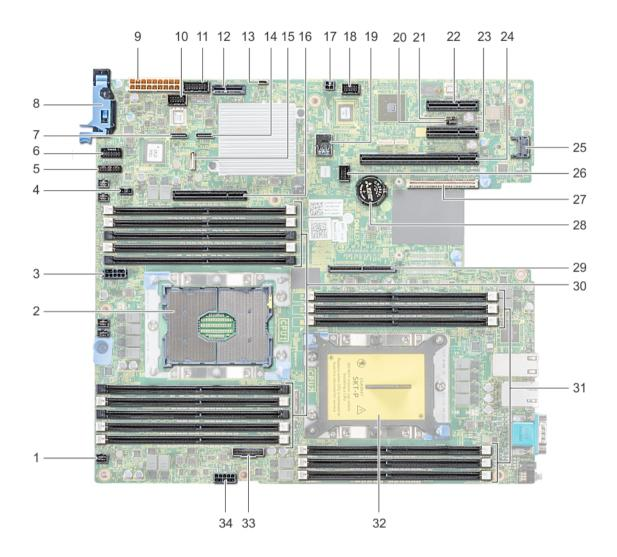
Figure 122. System board jumpers and connectors
