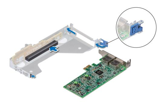
Figure 69. Installing expansion card into low profile riser
