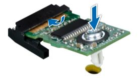
Figure 121. Installing the TPM
