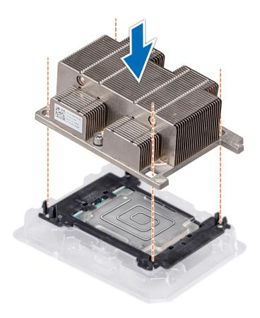
Figure 58. Installing the heat sink onto the processor
