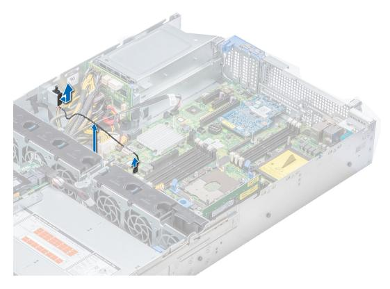
Figure 38. Removing an intrusion switch
