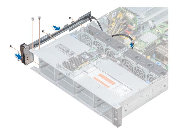
Figure 115. Installing left control panel
