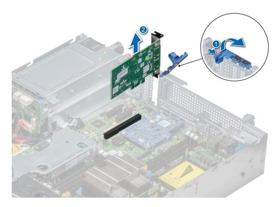
Figure 72. Removing expansion card from system board
