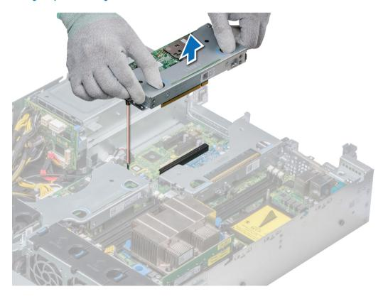
Figure 77. Removing low profile riser left
