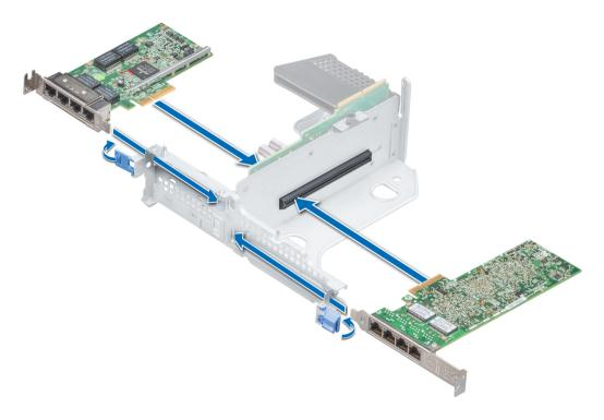
Figure 71. Installing expansion card into butterfly riser
