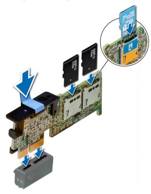
Figure 85. Installing optional IDSDM/vFlash card
