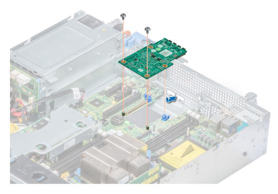
Figure 87. Installing LOM riser card
