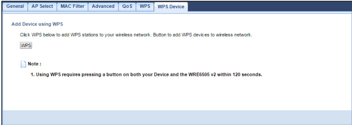
**Figure 40** Network > Wireless LAN 2.4G/5G > WPS Device (AP Mode)
