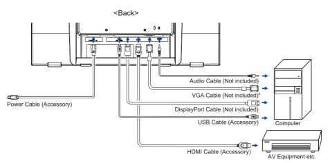
\* VGA cable is not supplied with the monitor. If you use low quality VGA cable, it may cause a result of electro-magnetic interference. Please contact the iiyama Support Centre in your country if you wish to connect the monitor via the VGA input.
