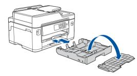
Pull the paper tray completely out of the machine as shown by the arrow. Take off the tray top cover.
