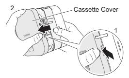
2. Insert the Tape Cassette following the drawing marked inside the case. Confirm that the tape is aimed at the green Tape Outlet and gently press the Tape Cassette into your machine until it locks into place.
