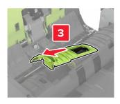
**4** Remove the ADF separator roller.
