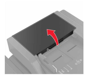
**3** Remove the ADF separator roller cover.
