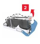
**4** Insert the new cartridge into the cartridge holder.
