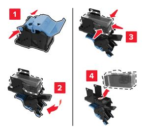
Insert the new cartridge into the cartridge holder.
