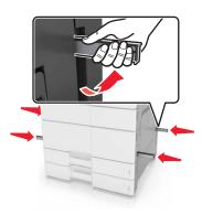
7 Align the printer with the tray, and then lower the printer into place.
