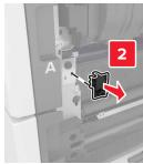
Loosen the screws of the transfer module lock.
