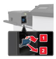
Remove the empty staple cartridge from the cartridge holder.
