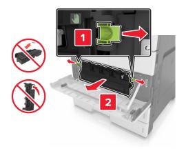
**3** Unlock the photoconductor unit.
