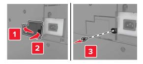
**12** Connect the power cord to the printer and electrical outlet.
