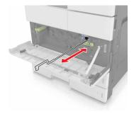
Remove the printhead wiper.
