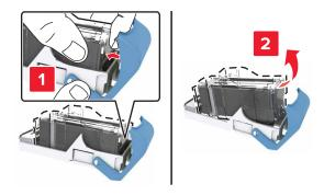
Insert the new cartridge into the cartridge holder.
