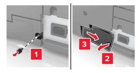
Remove the screws from the controller board access cover.
