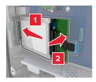
**b** Use the two provided screws to attach the hard disk mounting bracket.
