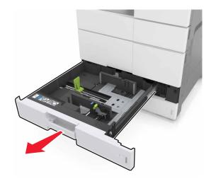
2 Squeeze and slide the paper guides to the correct position for the size of the paper you are loading.
