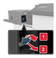
**4** Use the metal tab to lift the staple guard, and then remove any loose staples.
