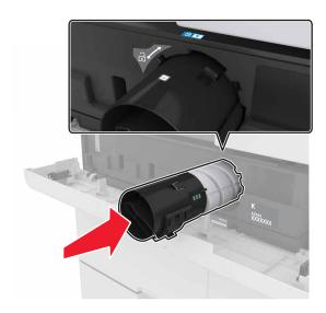
Rotate the cartridge clockwise to lock it into place.
