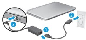
Your computer has a preinstalled battery. Before you press the power button to turn on the computer for the first time, be sure that the AC adapter is connected to the computer.
