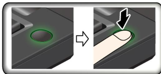
When the fingerprint reader indicator is solid green, tap your finger on the fingerprint reader for authentication.
