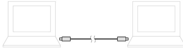
**Note:** The actual charging speed using the Lenovo-unique P-to-P 2.0 charging function varies depending on many factors, such as the remaining battery power of the computers, the wattage of the ac power adapter, and whether you are using the computers.
