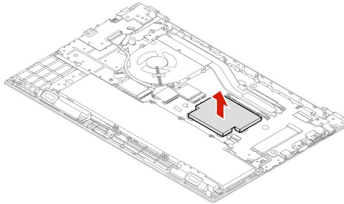
6. Open the latches on both sides of the memory module slot at the same time **1**, and then remove the memory module **2**.
