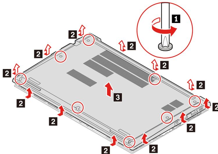
5. Install the new base cover assembly in place **1**. Ensure that the latches of the base cover assembly are secured under the base cover assembly **2**. Then, tighten the screws to secure the base cover assembly **3**.
