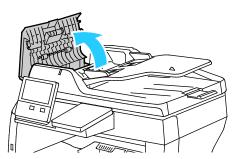
2. With a clean, lint-free cloth that is moistened with water, wipe the feed rollers and the separation pad until they are clean.
