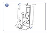
Rotate the machine to the horizontal position.
