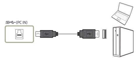
Connect the USB cable to 🕒 on the back of the product and USB 💳 on the PC.
