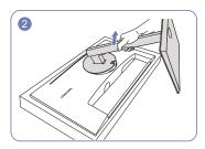
Lift the stand neck in the arrow direction to detach Unfasten the connecting screw at the bottom of the it from the display.
