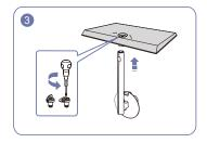
stand base, and then remove the stand neck from the stand base by pulling it in the arrow direction, as shown in the figure.
