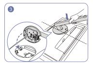
Place the stand neck on the display, as shown in the figure. When you place the stand neck, ensure that the two guides on the stand neck can be inserted into the groove of the display. Then press the stand neck downwards until the raise button on the stand neck insert into the groove of the display.
