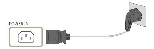
To use the product, connect the power cable to a power outlet and the POWER IN port on the product.
