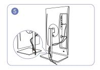
Place the corresponding cables into the stand-neck holder. Do not stretch the line. Three cables in one holder is recommended.
